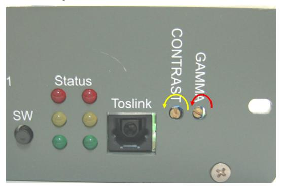
We can see the panel, there is two little pot, one for contrast adjustment (need professional person to do this), another one use for gamma level adjustment. Below is adjustment way:
