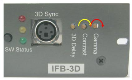
There are three little pots on the panel, one for contrast adjustment (need professional person to do this), and another one use for gamma level adjustment. Below is adjustment way:
