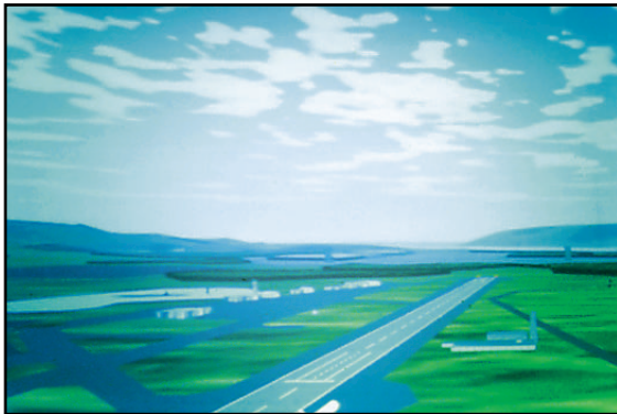
Figure 1 : The laws of physics applied to projection optics dictate that the center of the projected image will be brighter than the corners, a phenomenon normally referred to as 'corner fall off'.
